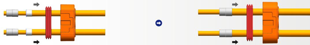
⑤ 接线端子剥线,剥线尺寸6mm,然后铆压
