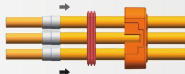
⑤ 接线端子剥线.剥线尺寸6mm.然后铆压
